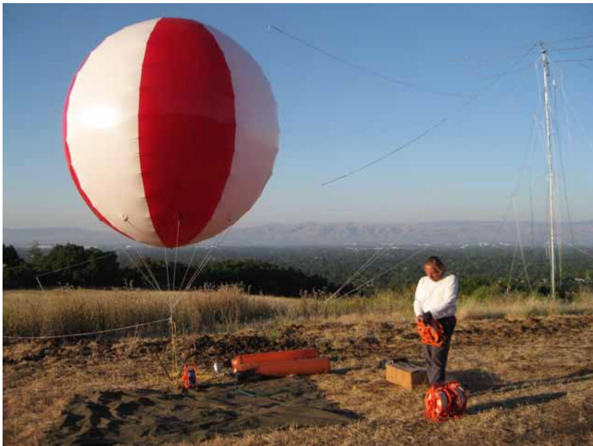
Svend (KF6EMB) deployed a helium balloon-supported full-wavelength loop antenna on 80 meters. This antenna is based on WU0I's award-winning QST article from July 2007, and give new meaning to that old 5 th Dimension song from the 1960s: "Up, Up and Away with my Beautiful Balloon."
